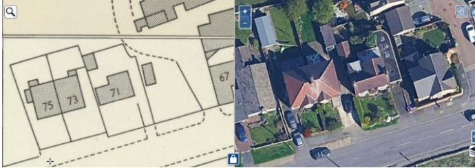
Figure 1 - Historic mapping and later aerial imagery Illustrates the apparent difference between the earlier dwelling footprint and the substantially enlarged building now occupying the site. Not relied upon as a measured survey.
